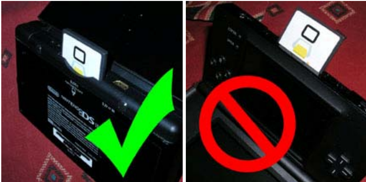
The correct and incorrect way of inserting the EZV.
