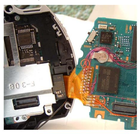
10. Bring the PSP motherboard into position and press down to connect it to the memory stick daughterboard via the plastic connector. Depending on the PSP hardware version the FPC cable may be obstructed at this point
