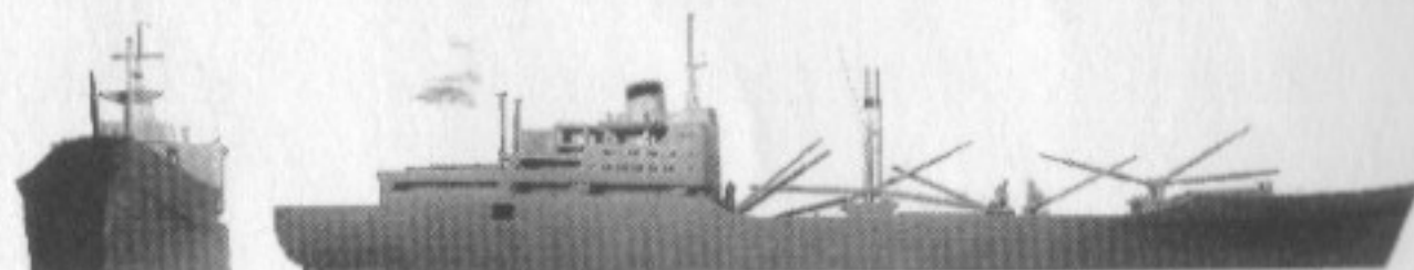
CARGO LINERS: Displ. 10,000-12,000 Tons LoA 560' Haw 128' SP 24k
